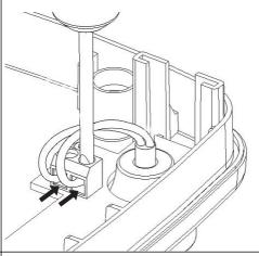
3 Secure the cable with the clamp
